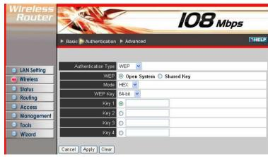
**WEP:** Open System allows public access to the router via wireless communications; Shared Key requires the user to set a WEP key to exchange data with other wireless clients that have the same WEP key.
